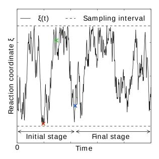
Fig. 5.40: AWH evolution in time for a Brownian particle in a double-well potential. The reaction coordinate  $\xi(t)$  traverses the sampling interval multiple times in the initial stage before exiting and entering the final stage. In the final stage, the dynamics of  $\xi$  becomes increasingly diffusive.
