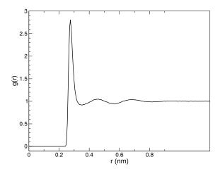
Fig. 5.53:  $g_{OO}(r)$  for Oxygen-Oxygen of SPC-water.
