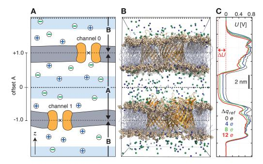
Fig. 5.48: Typical double-membrane setup for CompEL simulations (A, B). Ion/water molecule exchanges will be performed as needed between the two light blue volumes around the dotted black lines (A). Plot (C) shows the potential difference  $\Delta U$  resulting from the selected charge imbalance  $\Delta q_{ref}$  between the compartments.
