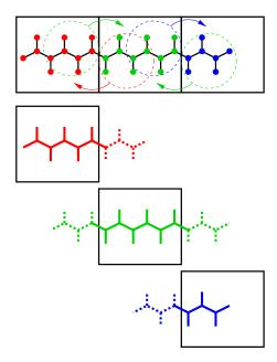
Fig. 5.13: Example of the parallel setup of P-LINCS with one molecule split over three domain decomposition cells, using a matrix expansion order of 3. The top part shows which atom coordinates need to be communicated to which cells. The bottom parts show the local constraints (solid) and the non-local constraints (dashed) for each of the three cells.
