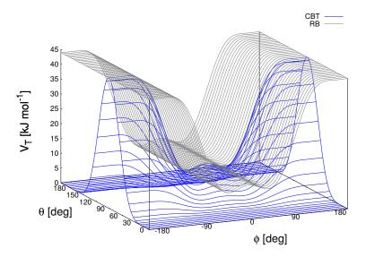
Fig. 5.28: Blue: surface plot of the combined bending-torsion potential ((5.182) with k=10 kJ mol<sup>-1</sup>,  $a_0=2.41$ ,  $a_1=-2.95$ ,  $a_2=0.36$ ,  $a_3=1.33$ ) when, for simplicity, the bending angles behave the same ( $\theta_1=\theta_2=\theta$ ). Gray: the same torsion potential without the  $\sin^3\theta$  terms (Ryckaert-Bellemans type).  $\phi$  is the dihedral angle.
