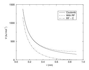
Fig. 5.18: The Coulomb interaction (for particles with equal signed charge) with and without reaction field. In the latter case  $\varepsilon_r$  was 1,  $\varepsilon_{rf}$  was 78, and  $r_c$  was 0.9 nm. The dot-dashed line is the same as the dashed line, except for a constant.
