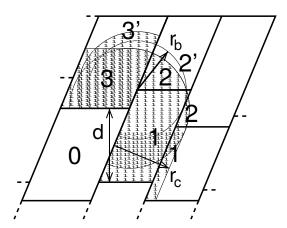
Fig. 5.12: The zones to communicate to the rank of zone 0, see the text for details.  $r_c$  and  $r_b$  are the non-bonded and bonded cut-off radii respectively, d is an example of a distance between following, staggered boundaries of cells.
