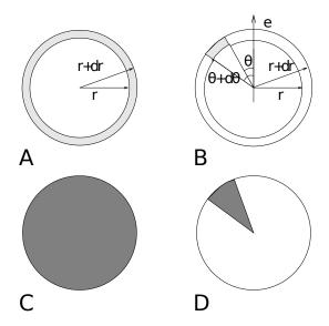
Fig. 5.52: Definition of slices in gmx rdf (page 135): A.  $g_{AB}(r)$ . B.  $g_{AB}(r,\theta)$ . The slices are colored gray. C. Normalization  $\langle \rho_B \rangle_{local}$ . D. Normalization  $\langle \rho_B \rangle_{local}$ ,  $\theta$ . Normalization volumes are colored gray.
