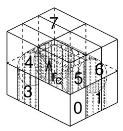
Fig. 5.11: A non-staggered domain decomposition grid of  $3\times2\times2$  cells. Coordinates in zones 1 to 7 are communicated to the corner cell that has its home particles in zone 0.  $r_c$  is the cut-off radius.
