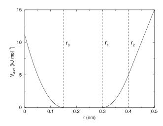
Fig. 5.31: Distance Restraint potential.
