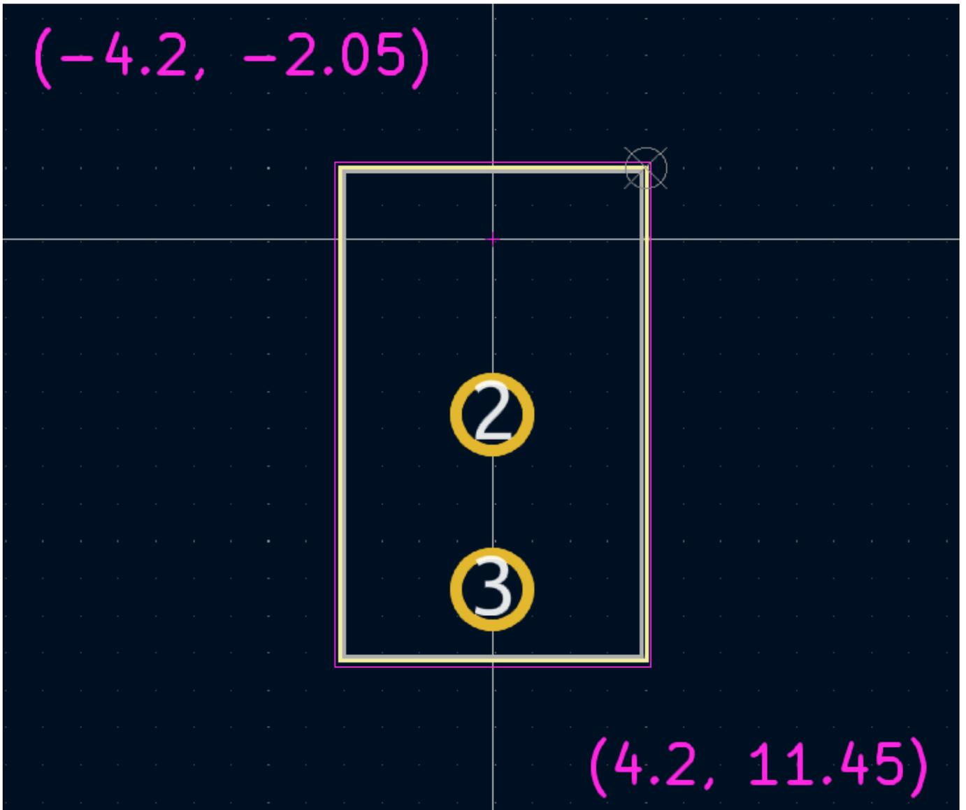
After completing the outlines, position the text as shown below. The footprint is complete.
