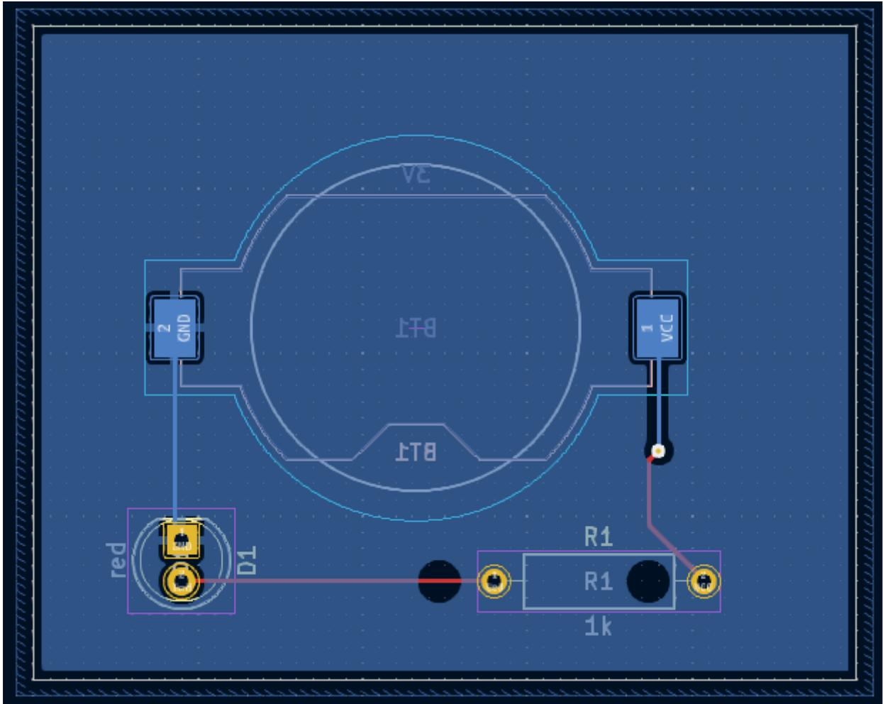
Run DRC again, but make sure to uncheck the *Refill all zones before performing DRC* checkbox. DRC reports 4 violations: for each pad of R1, there is a clearance violation between the pad and the zone and another clearance violation between the pad's through hole and the zone. Arrows point to each violation in the canvas. Clicking on each violation message zooms in on the respective violation.
